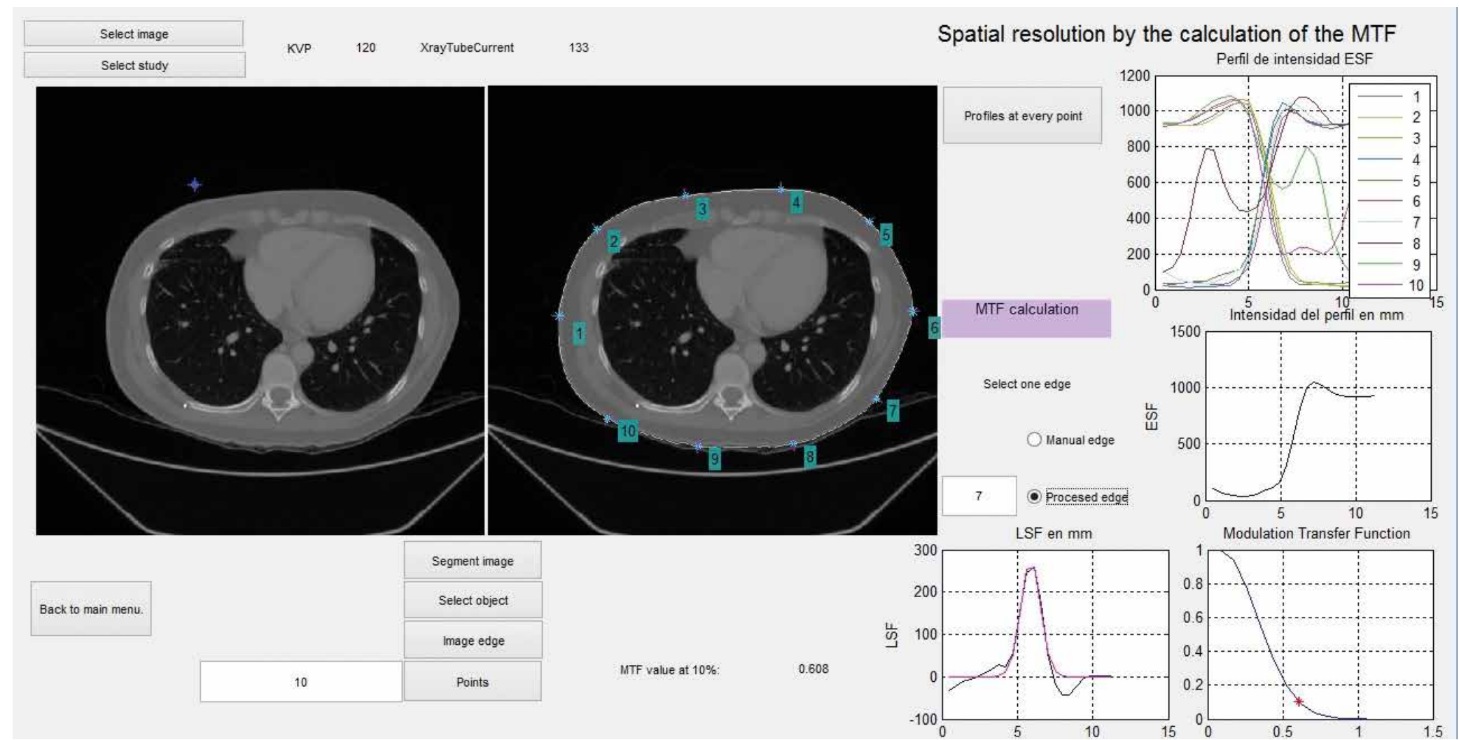
Fig. 1: Screenshot of the software developed to calculate noise and spatial resolution
