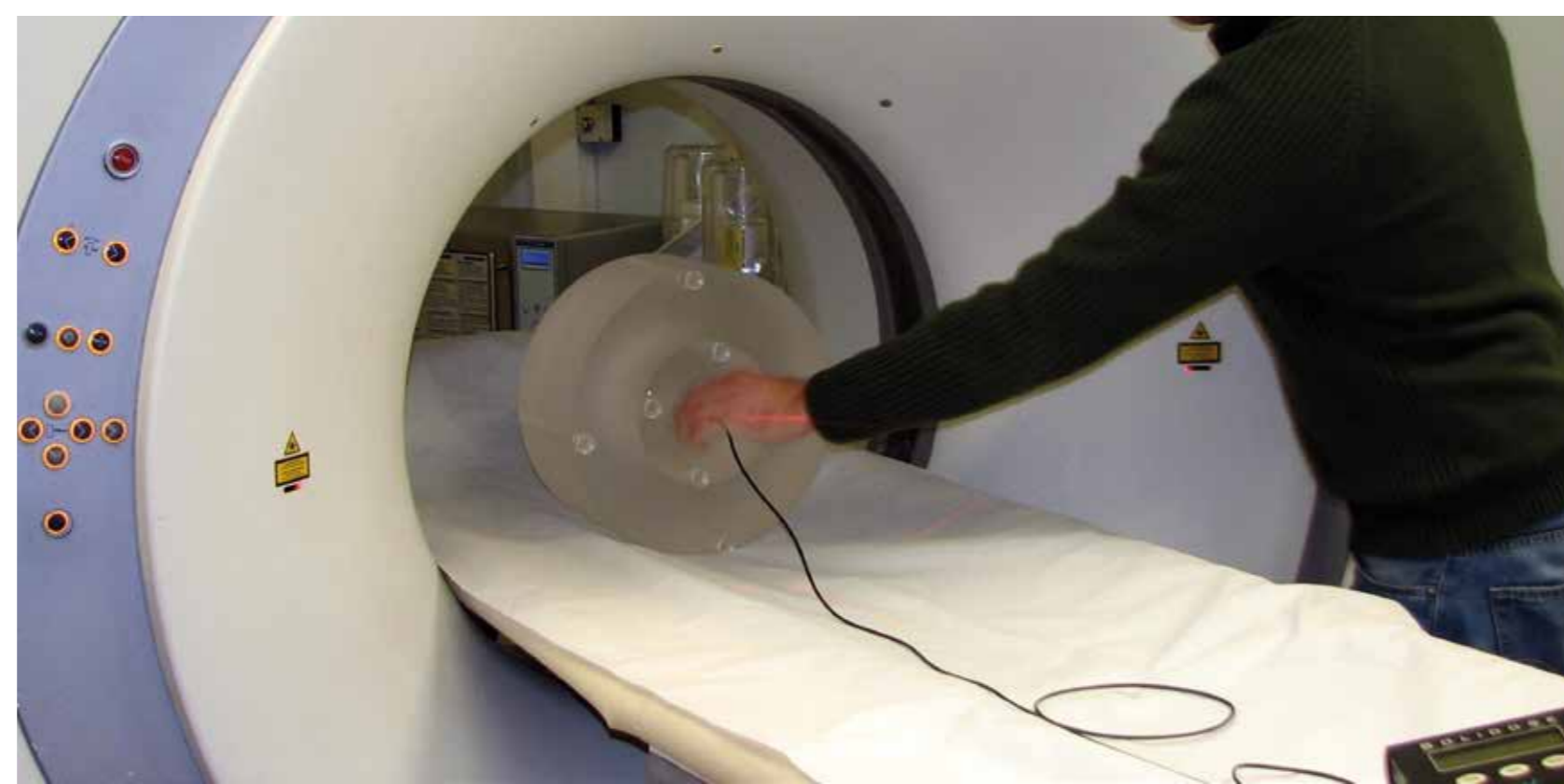
Fig. 1: CTDI measurement using a phantom and a pencil ionization chamber.
