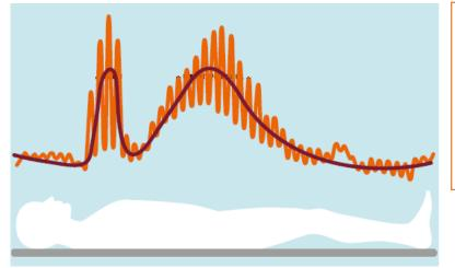
Angular tube current modulation changes the mA during the rotation (xy-axis). For the shoulders, the tube current increases laterally but decreases in the PA/AP projections.
