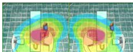
Optimising staff exposure: isodose maps and x-ray tube position
